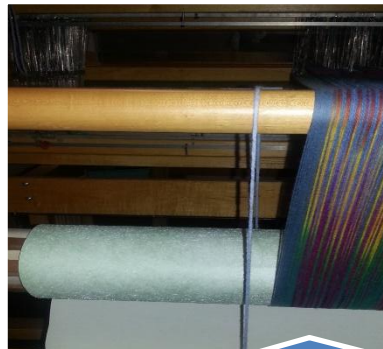
This is a closeup of the tieup on the back beam and how it rolls
