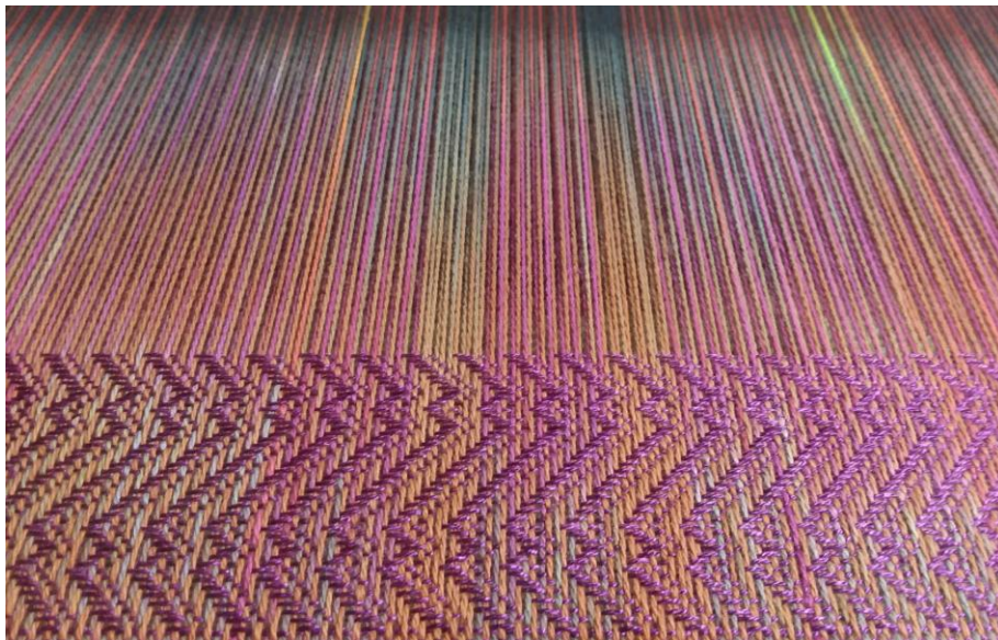
The warp is a combination of 2 Blazing Shuttles 8/2 cotton dyed warps, Autumn Mead & Autumn Leaves & the weft is 8/2 tencel Red Purple. The 8-S draft is #315-1 from Stricklers book.
